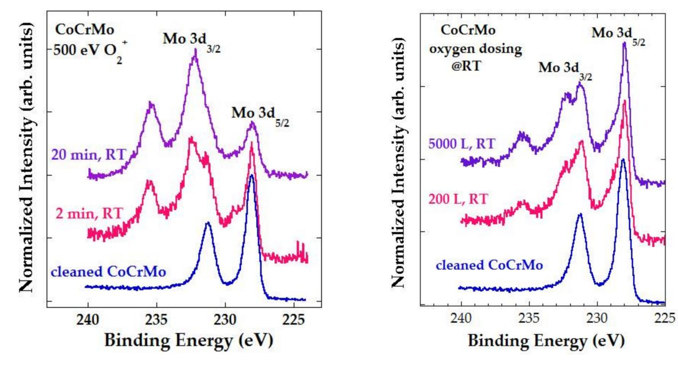
The photoemission spectra taken on the cleaned CoCrMo surface and surfaces oxidized by ion bombardment for two different bombardment times (left) and with two different oxygen doses (right).
