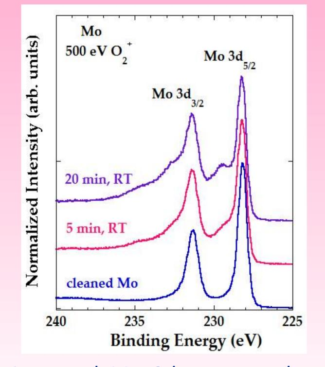
A several Mo 3d spectra taken from a cleaned Mo surface and surfaces bombarded with 500  $eV O_2^+$  ions for two different bombardment times of 5 and 20
