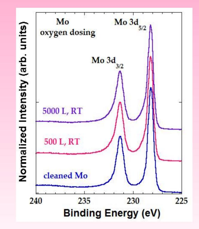
Mo 3d core-level photoemission from cleaned spectra а molybdenum surface and surfaces after oxidation at room temperature (RT), with oxygen
