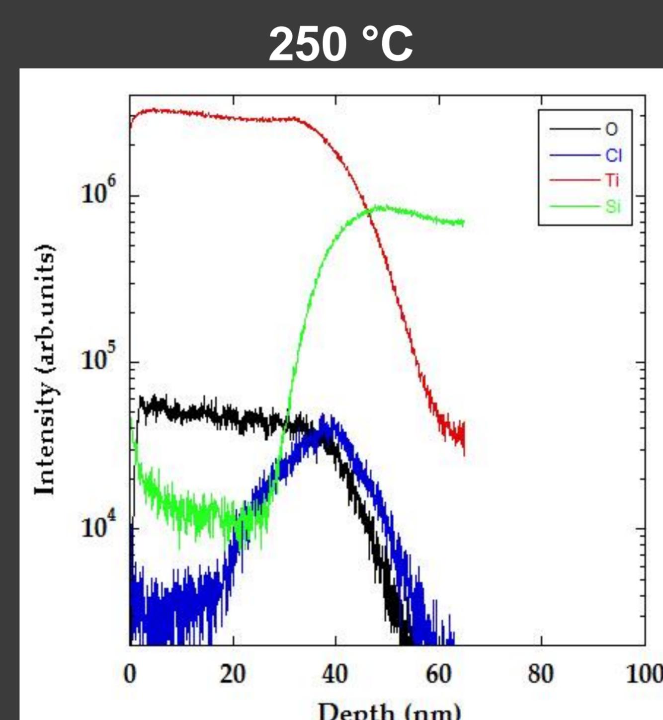
**SIMS depth profiles** at TiO<sub>2</sub> films grown on 40 °C and 250 °C using plasma-enhanced ALD. Spectra were recorded by measuring positive ions of Ti and Si (using 3 keV O<sub>2</sub><sup>+</sup> primary ions), and negative ions of O and Cl (with 5 keV Cs<sup>+</sup> primary ion beam).
