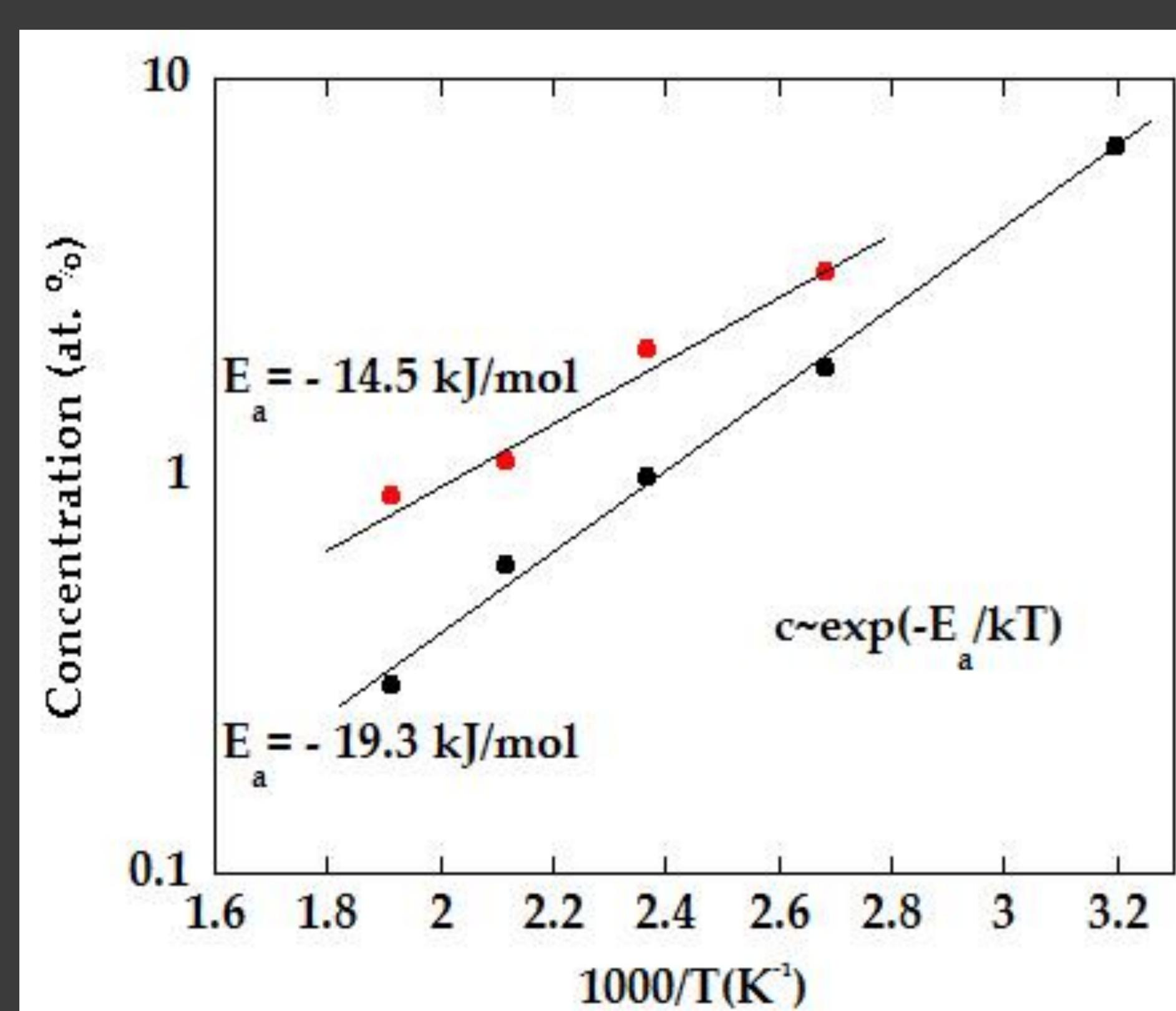
**Arrhenius plot** of Cl concentration vs reciprocal temperature ( $1000/T$ ) for samples grown by thermal ALD and PEALD. The linear fitted lines were used to calculate the activation energy.
